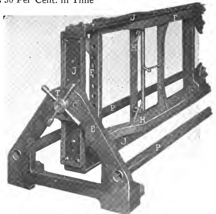
National frame in jig placed beneath the radial drills. When one side is drilled the jig can be rotated with the frame
